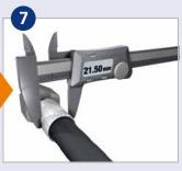
Check the crimp results at multiple points. If necessary, adjust the machine setting to reach the required crimp diameter value.
