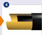
Pay attention to internal and external skive lengths and remove all visible rubber to the correct marks. Ensure wires are not damaged. After skiving ensure ALL surfaces are clean.
