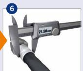
Check the crimp results at multiple points. If necessary, adjust the machine setting to reach the required crimp diameter value.
