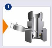
**Attention!** Stainless steel threads must be lubricated (ABF grease)
