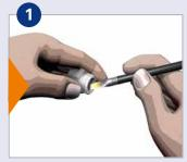
**Attention!** stainless steel threads must be lubricated (ABF grease)
