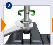
Assemble fitting until wrench tight (without spanner extention)
