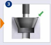
Check for deformation of geometry
