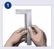
**1. Saw the tube off square.** An angular deviation of 0,5° relative to the tube axis is permissible.
