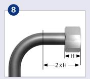
8. Minimum length of straight tube end for tube bends
