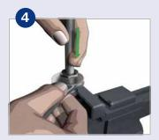
**4. Find point of resistance** Push pipe completely into the connector. Tighten nut until the ring makes contact with the tube surface – this point can be felt by an increase in torque.
