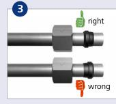
**3. Assembly of cutting ring** Place nut and cutting ring on tube as shown.
